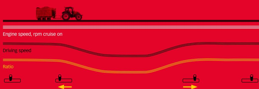
Manual mode can be selected in A and B work areas. The transmission ratio is controlled solely by driver using the CVT lever. Suitable especially for harvesting tasks that require specific speeds for different conditions and crops.
