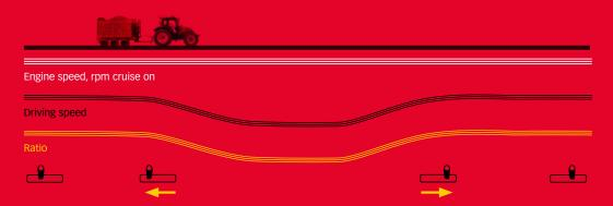
Manual mode can be selected in A and B work areas. The transmission ratio is controlled solely by driver using the CVT lever. Suitable especially for harvesting tasks that require specific speeds for different conditions and crops.
