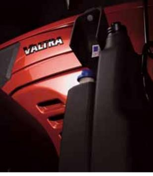
Valtra and AGCO Sisu Power have been a strong team for more than 50 years. Together we have introduced many world-class innovations over the decades. The new AGCO Sisu Power SCR engines are also clearly ahead of their time and offer unmatched levels of efficiency. SCR technology uses urea based AdBlue to reduce exhaust emission, the SCR technology is already being used in heavy trucks. Already today they comply with Tier 3B emissions standards for 2011.
